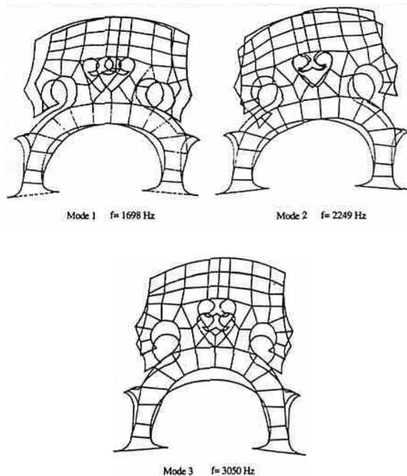
Figure 4. Standard cello bridge in-plane vibrating mode patterns.
