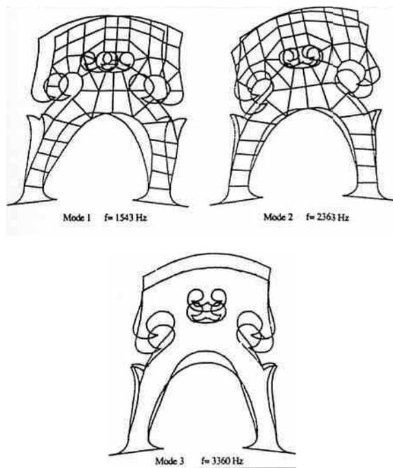
Figure 6. Belgian cello bridge in-plane vibrating mode patterns.
