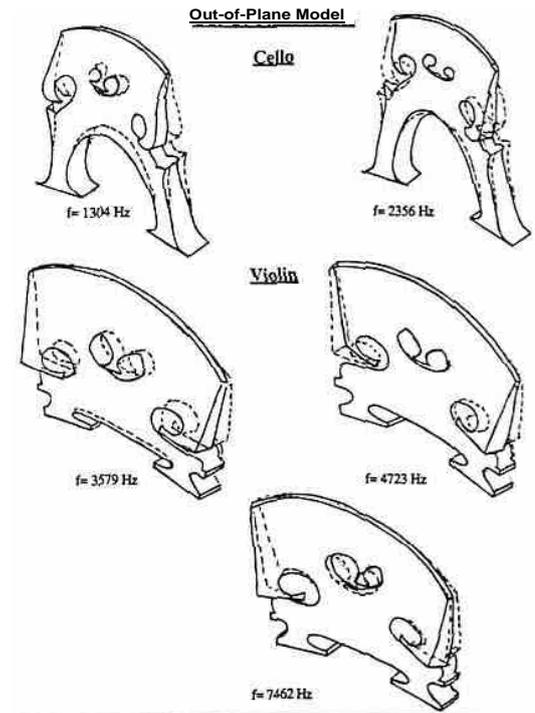
Figure 8. Out-of-plane vibrating mode patterns for all bridges.
