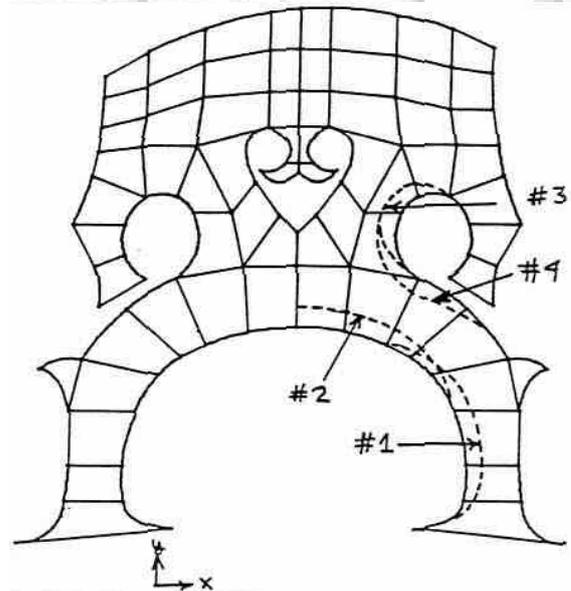
Figure 5. Cutout patterns for the standard cello bridge.
